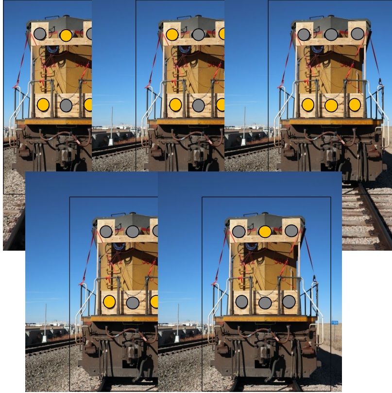
Figure 8. Rear of the locomotive depicting all lamp patterns tested
