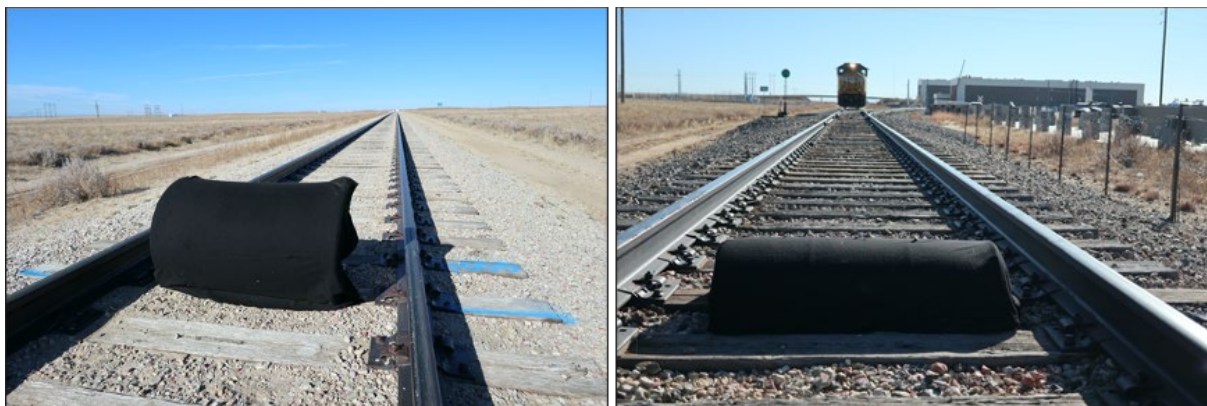
Figure 6. On-track targets at different visual angles placed on the test track
