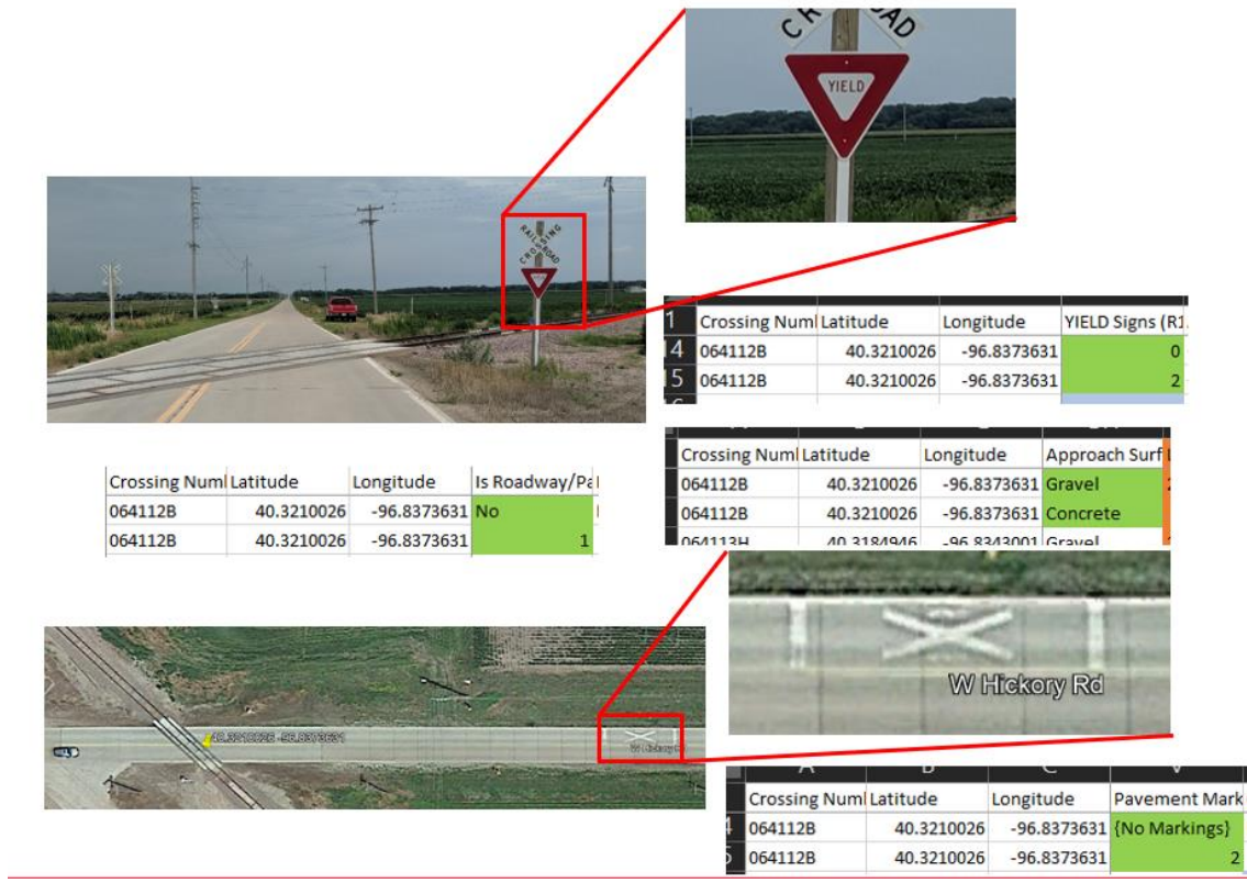
Figure 4.3 Data Correction Example, Crossing 064112B
