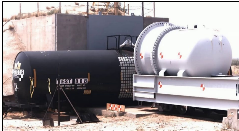
Figure 2. Still Frame from Shell Impact Test in 2018 of DOT-105 Tank Car (Test 8)
