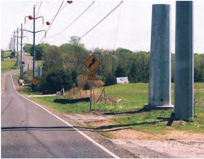
Figure 18. Example of utility poles (such as transmission poles) that cannot be relocated, requiring consideration of alternative treatments (Photo: Don Ivey).
