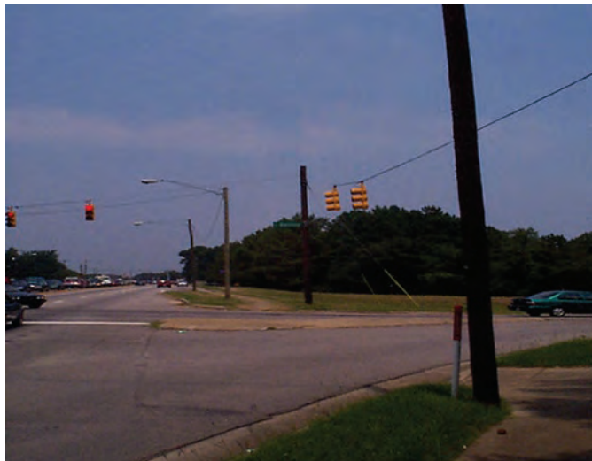
Figure 20. Example of a good candidate for safety improvement by burying utility lines (Photo: Charles Zegeer).
