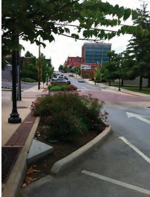
Figure 19. Example of a traffic-calming measure, with a narrowing road and pedestrian crossings (Photo: Kristen Brookshire).
