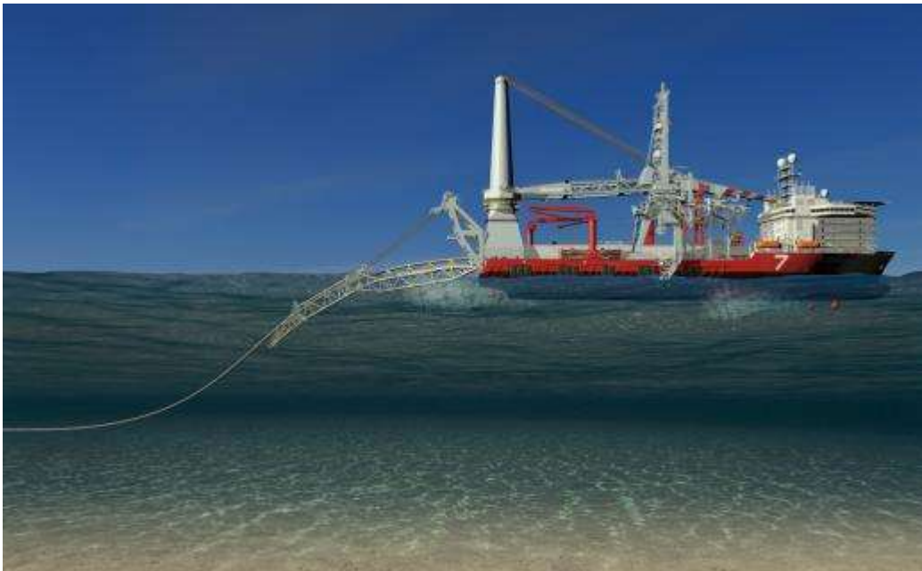
Figure 1: S-Lay Pipeline Installation Method
