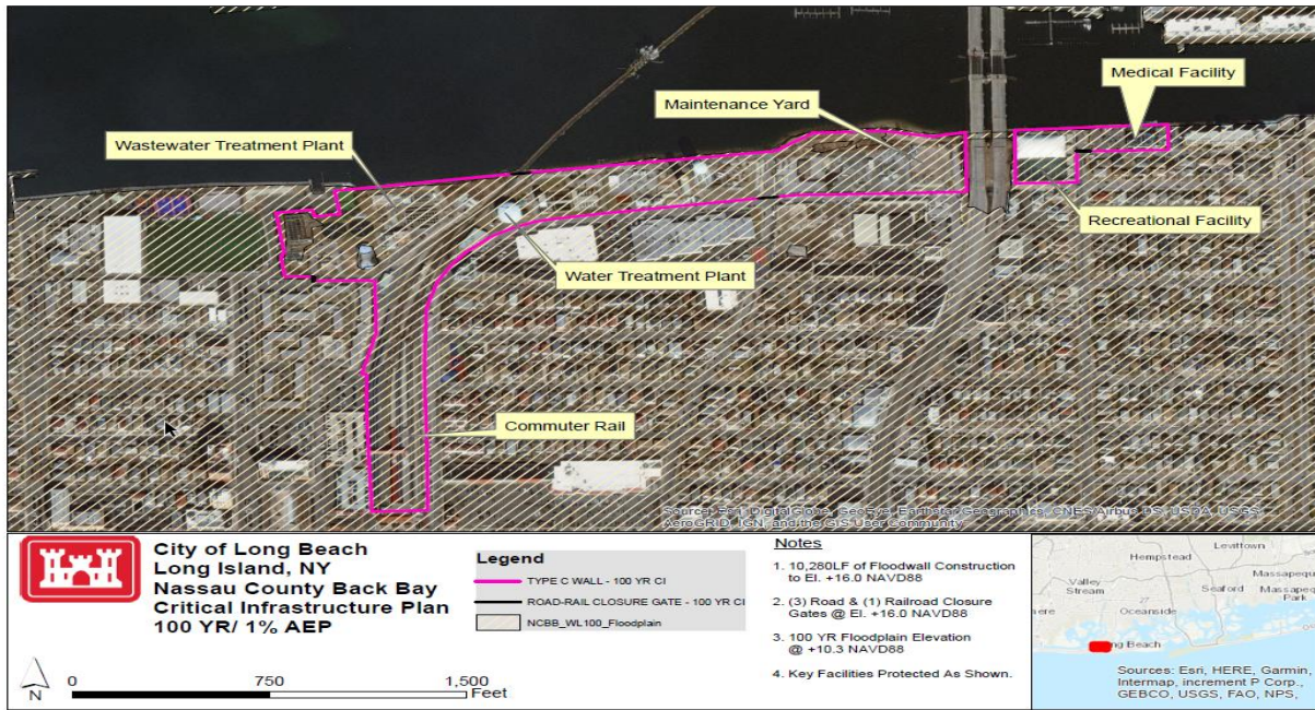
Figure 8: Local Floodwall in the City of Long Beach
