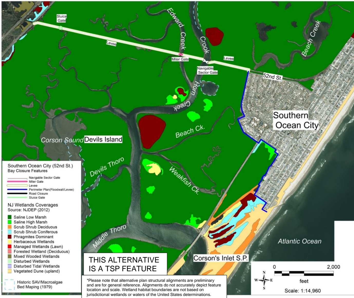
Figure 17. Interior Bay Closure Overlay with Wetland Habitats at Southern Ocean City in TSP Alternative 4G(8)
