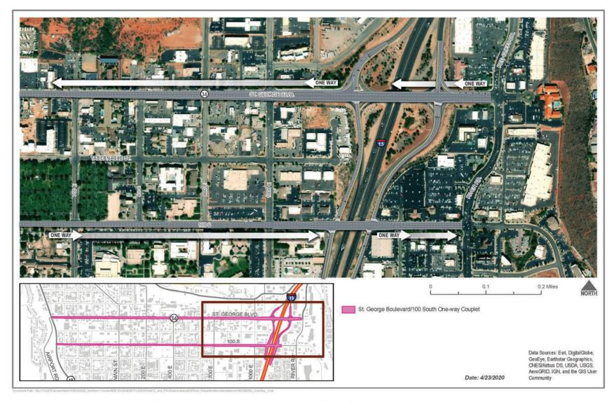
Figure 11c. St. George Boulevard/100 South One-way Couplet Plan View (3 of 4)
