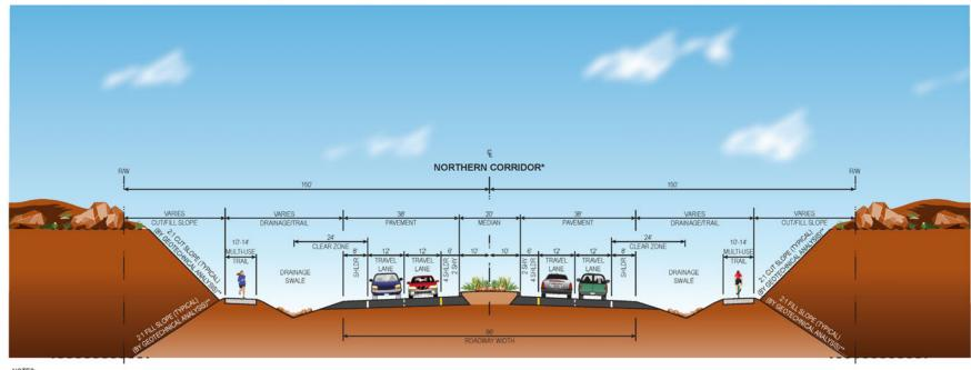
Figure 6. T-Bone Mesa Alignment, UDOT Application Alignment, and Southern Alignment – Highway Cross Section, Eastbound within the NCA
