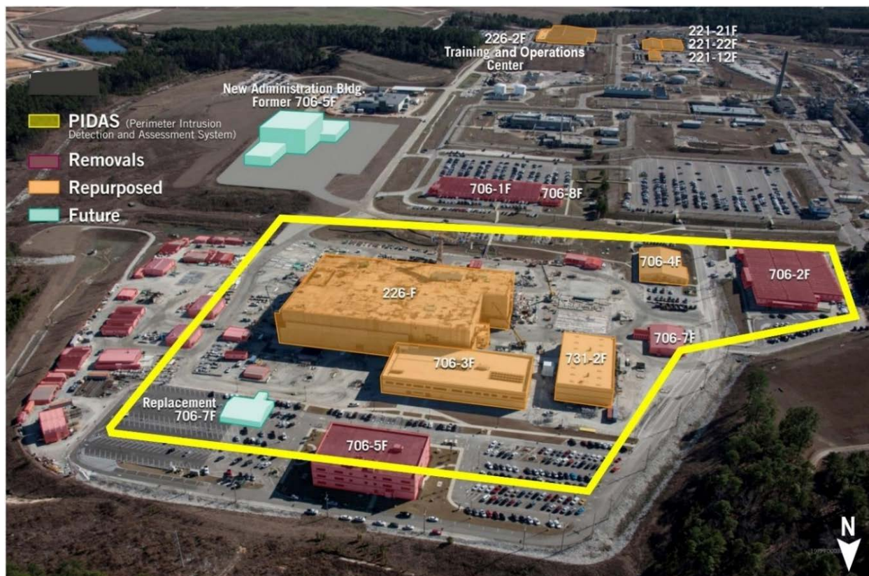
Figure 4-1—Proposed Layout Under the Proposed Action (showing facility removal, reuse, and new construction)
