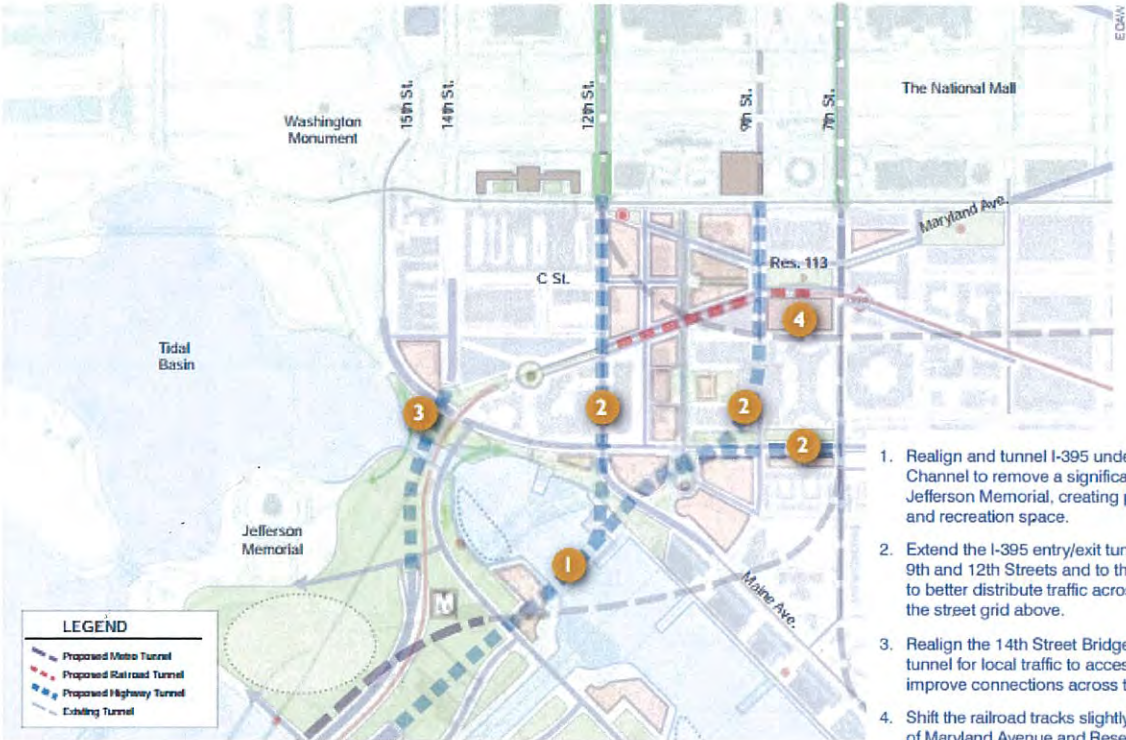
Diagram of proposed tunnels that could improve street-level development and connectivity.
