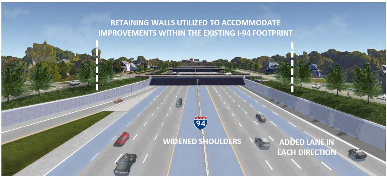
Figure 3-8: Approved Selected Alternative with Modifications Cross-Section
