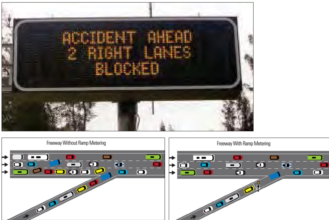
Figure 3-9: Dynamic Message Signs and Ramp Metering
