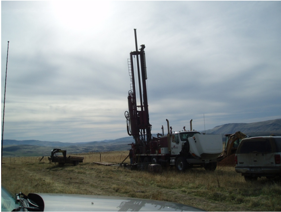
Figure 1. Temperature Gradient Drill Rig at Crane Creek, Fall 2009
