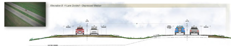
Figure 2: Typical Section for Divided, Depressed Median.
