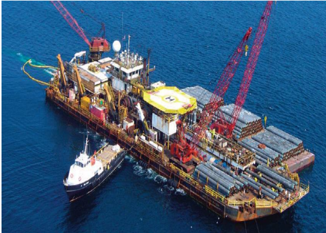
Figure 2.3.3-4 Typical Pipelay Barge
