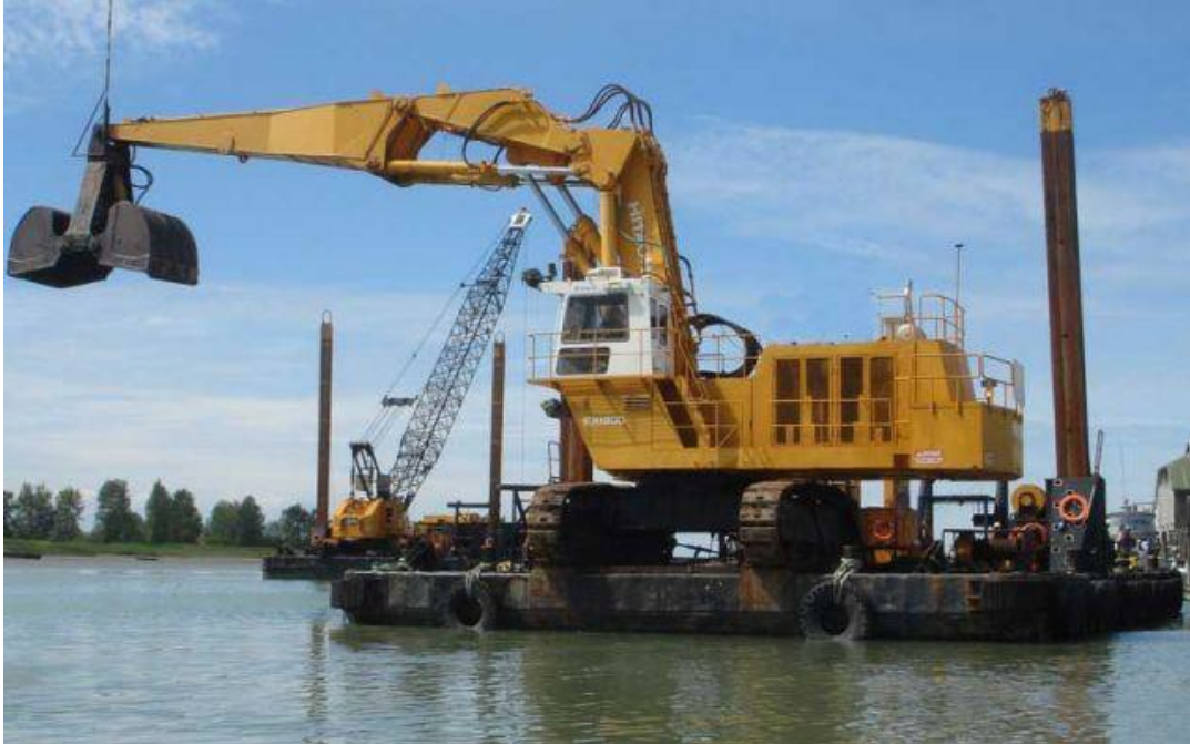
Figure 2.3.3-3 Typical Clamshell Barge
