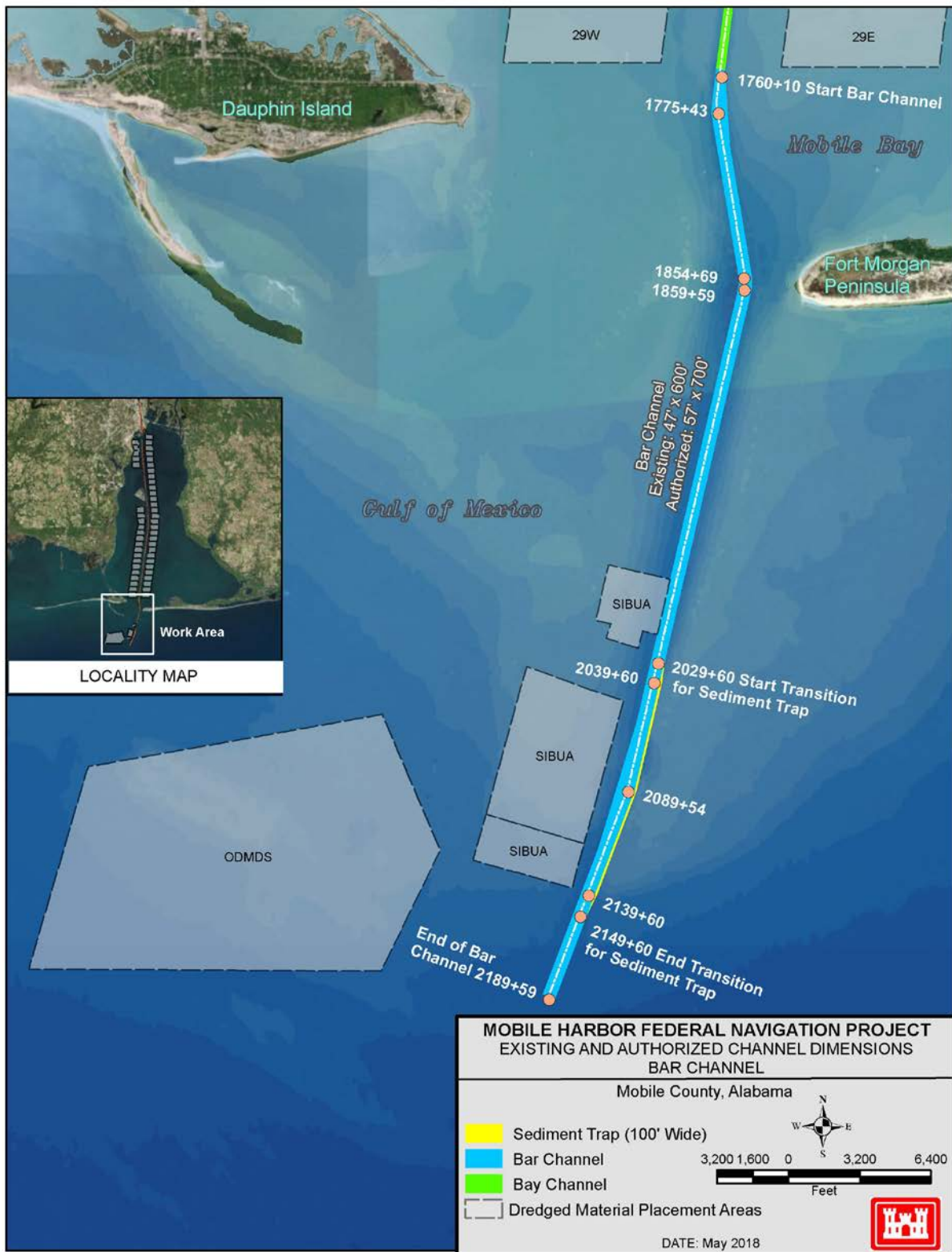
Figure 2-18. Bar Channel Alignment and Stationing
