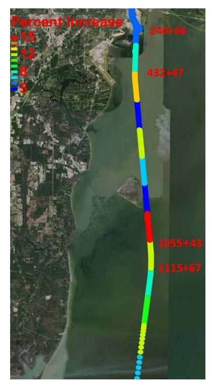
Figure 109. Simulated increases in annual shoaling vary from 5 to 15 % along channel with-Project depths. Four channel stations are shown in red to the east side of the channel.
