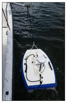
Figure 3: Sontek M9 Acoustic Doppler Current Profiler Field Deployment Configuration.
