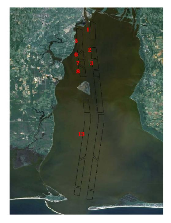
Figure 100. Placement Areas (black quadrilaterals) along the navigation channel. Number of Placement Area in red.
