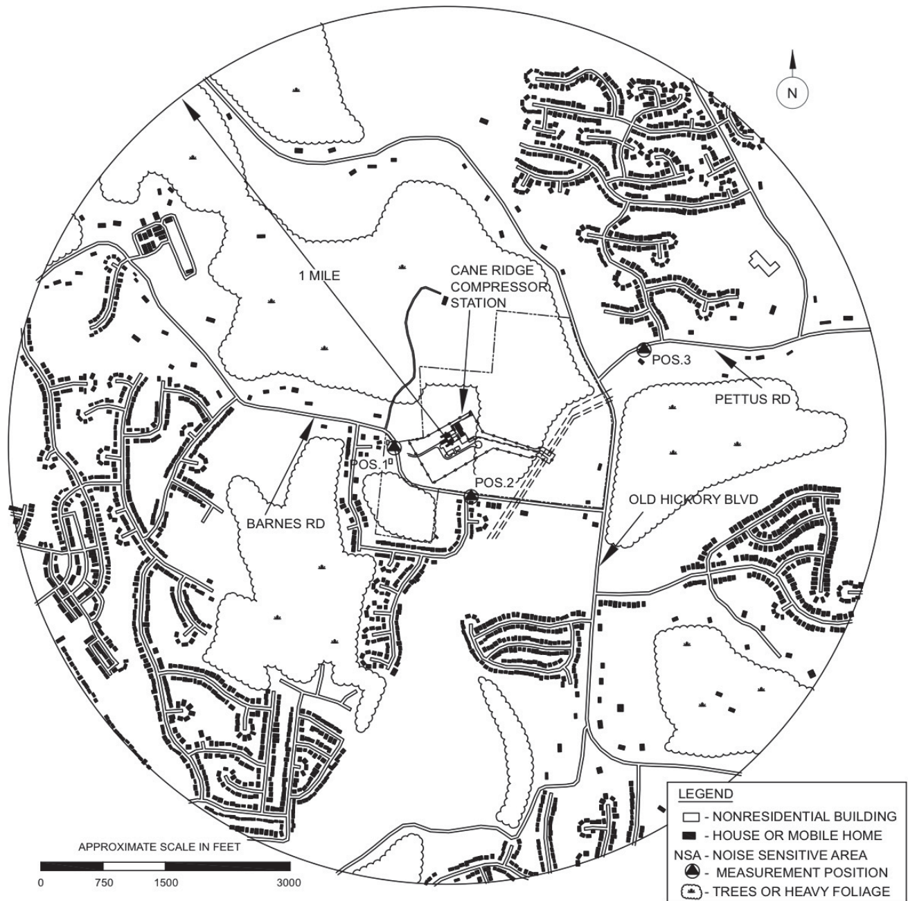
Figure 1: Cane Ridge Compressor Station (GXP Project): General Area Layout around the Station showing the NSAs within 1 Mile of the Station Site and Other Areas of Interest.
