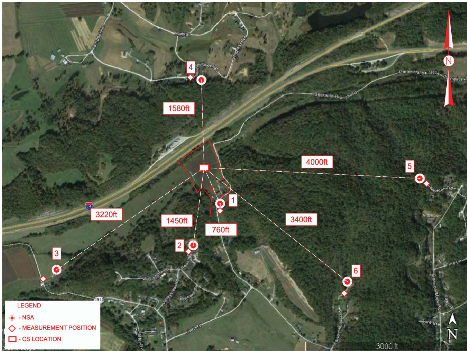
Figure A NSA Distances and Directions, Referenced from Proposed Compressor Building Location.
