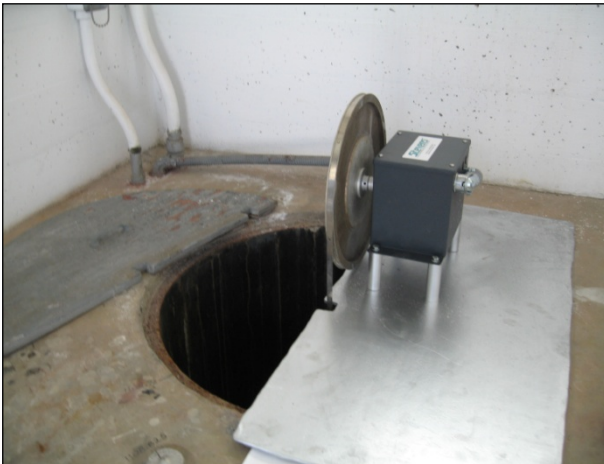
Figure 5-1. Encoder with Wheel Tape for Measuring the River Stage or Lake Elevation in a Stilling Well
