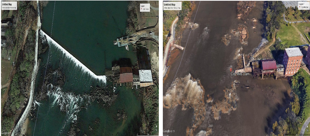
Figure 4-16. City Mills Dam Before and After Dam Removal (Photographs courtesy of Google Earth)
