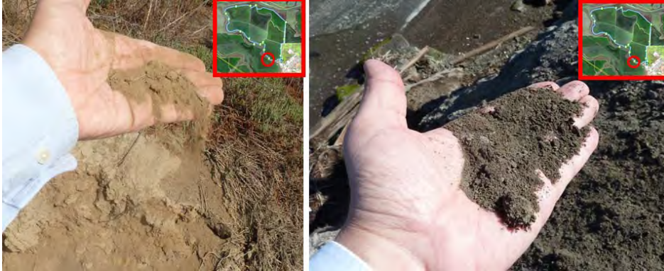
Figure 4 - Crest loose silt behavior with some to high organic fiber content
