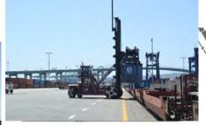
Containers loaded/unloaded to train cars at on-dock railyard
