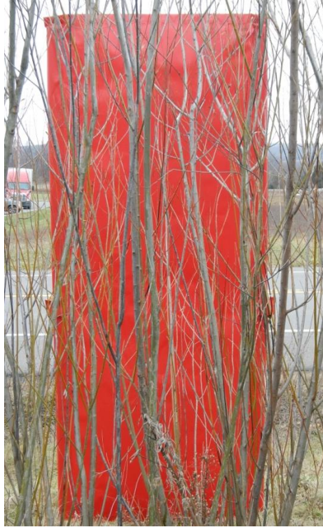
Figure 5: Picture taken of living snow fence Tully-B-willow-6 with a red chroma-key backdrop held behind the fence to create a strong color contrast and accurately sample optical porosity
