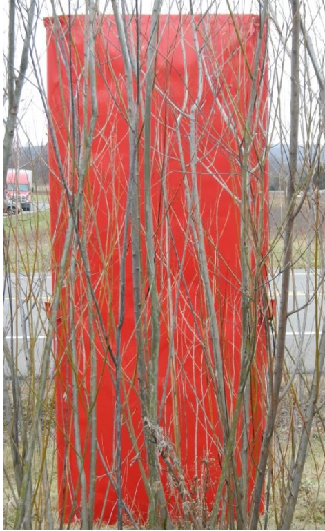
Figure 6: Chroma-key backdrop held in front of a shrub-willow living snow fence to create a contrast between fence vegetation and open space to photograph the fence and to measure the optical porosity
