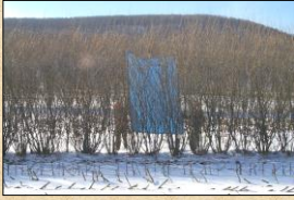
Measuring optical density on a living willow snow fence in Cortland County, NY
