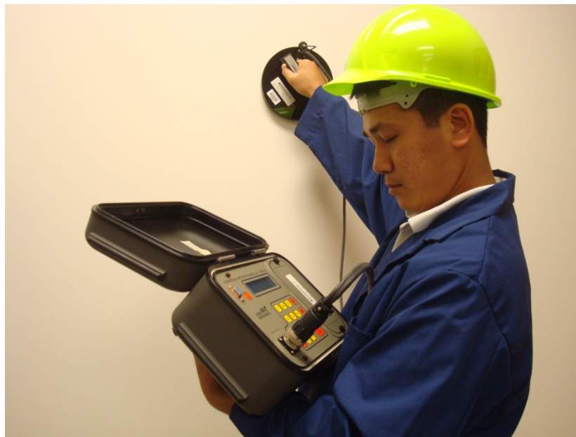
Figure 3.11 Gecor 6 Device with Sensor
