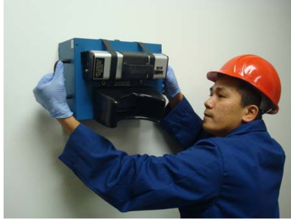
Figure 3.1: Installing the ASR-260 Field Inspection Kit
