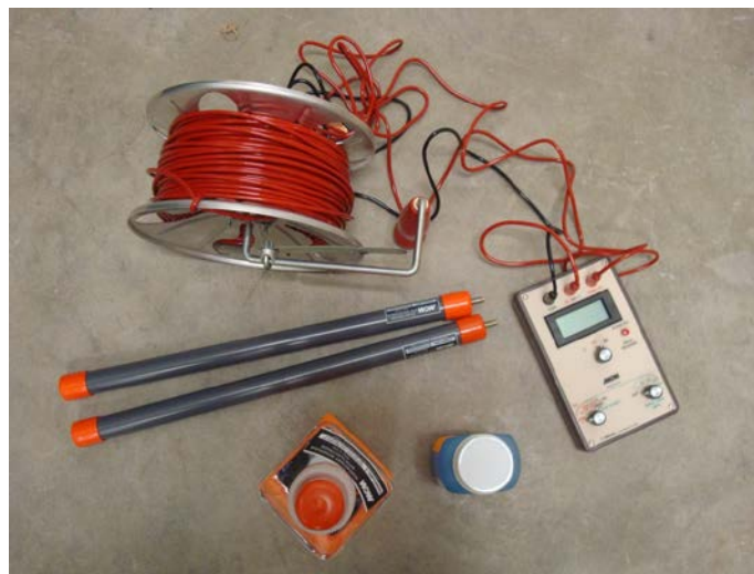
Figure 3.3 Devices for Electrode (half cell) Potential Measurements
