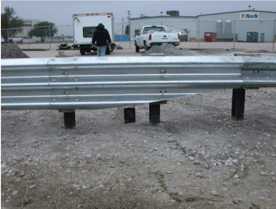
Figure 18. Asymmetric Transition Element for Test No. MWT-4 [21]
