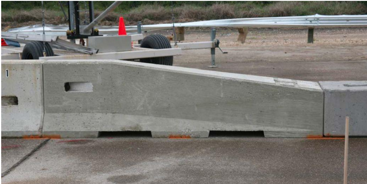
Figure 22. Low-Profile-to-F-Shape Transition Barrier Segment [25]
