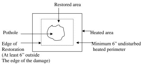
Figure D.1: Proper Heater Placement
