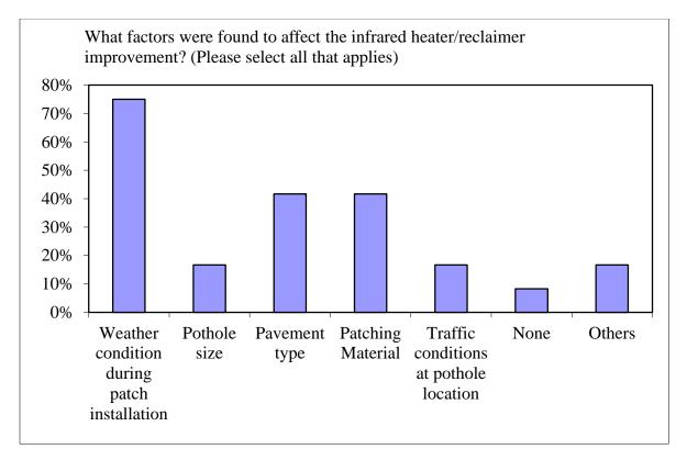
Figure 4.3 Factors Affecting Infrared Asphalt Heaters/Reclaimers Improvement
