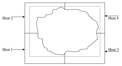
Figure D.2: Multiple Hit Heating Pattern For A Large Repair
