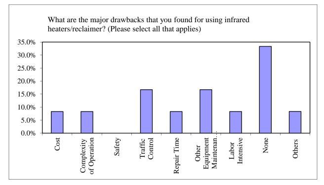
Figure 4.5 Main Drawbacks of Infrared Asphalt Heaters/Reclaimers
