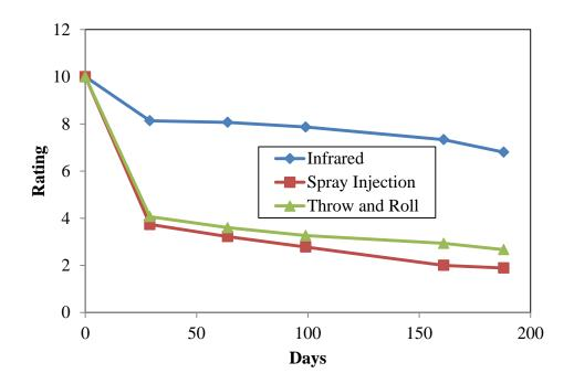
Figure 6.8 Overall Rating With Time For Each Patching Method
