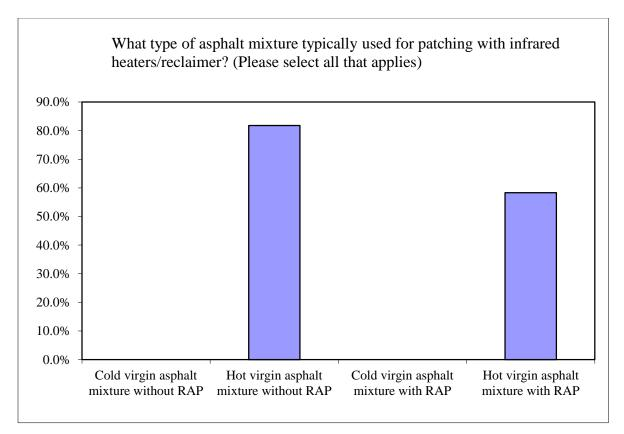
Figure 4.4 Type of Mixture Used for patching with Infrared Asphalt Heaters/Reclaimers
