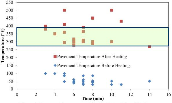
Figure 6.3 Pavement Temperatures Before And After Infrared Heating
