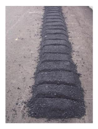
Figure 7.1 Example of Proper Storage Procedure for Asphalt Mixtures Used In Infrared Method
