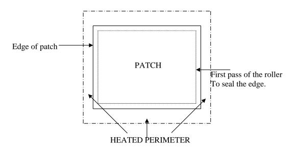
Figure D.3 Demonstration for Proper Compaction Procedure
