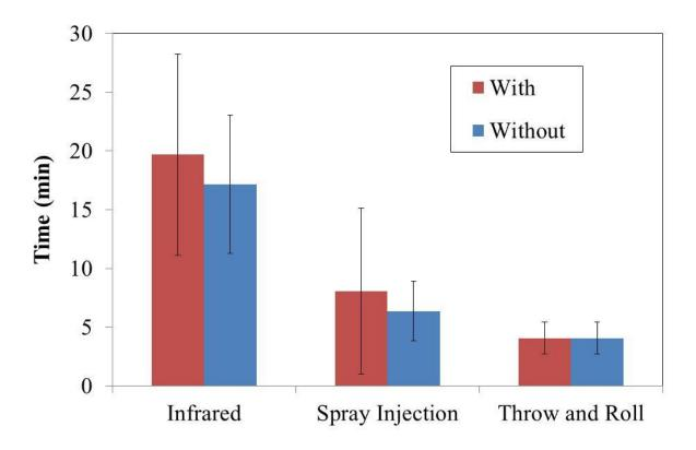
Figure 6.1Average Patching Duration of the Different Patching Methods with or without Patching Operation Encountered Problems
