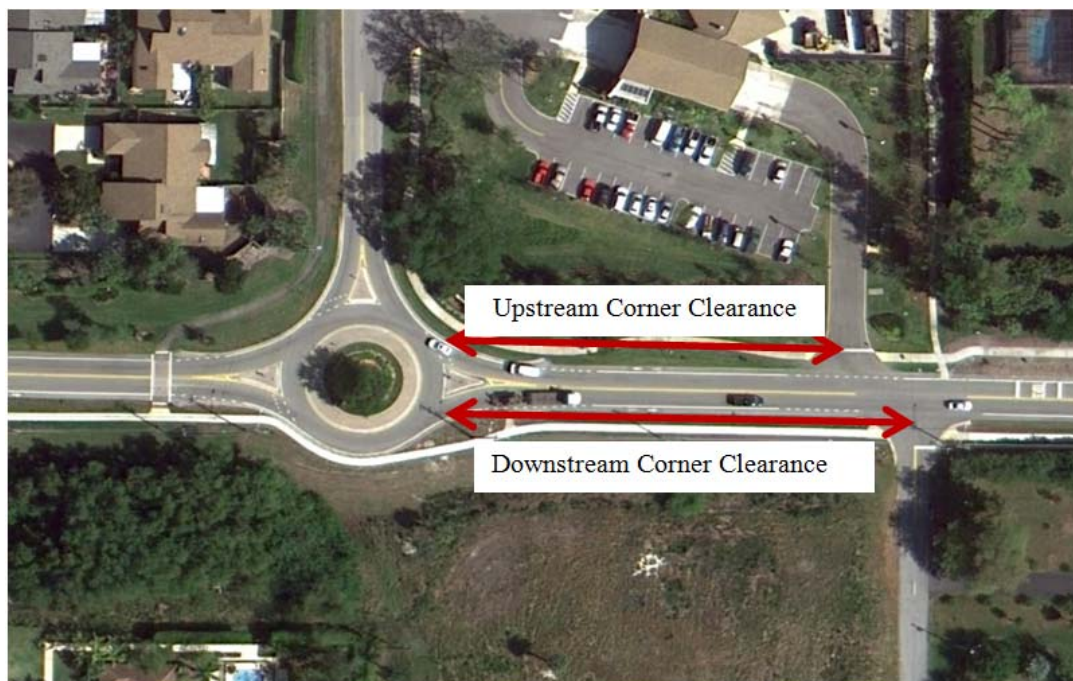
Figure 39. Upstream and Downstream Driveway Corner Clearances
