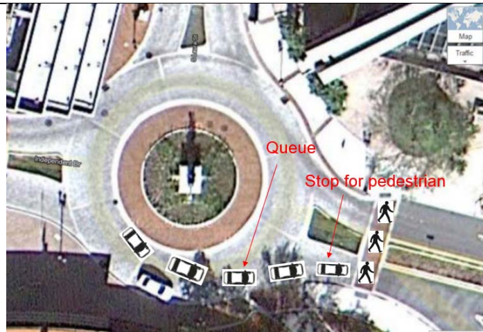
Figure 57. Roundabout Observation with Pedestrian Conflict (Independent Dr. and S. Laura St., Duval County)
