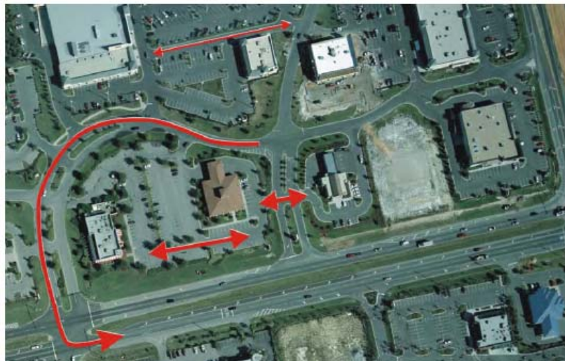
Figure 28. Joint and Cross Access (FDOT, 2008, p. 86)
