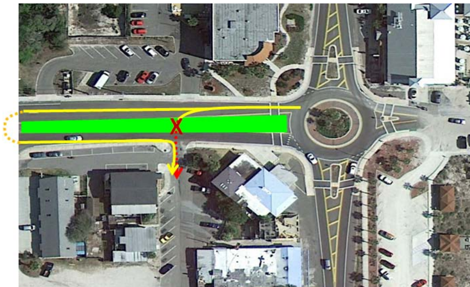
Figure 48. Closing Median Openings Prevent Vehicles From Turning Left From the Main Street Onto the Driveway
