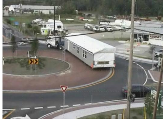
FIGURE 5.13a Long, Wide OSOW Making a Left Turn at Greenwich, NY Roundabout
