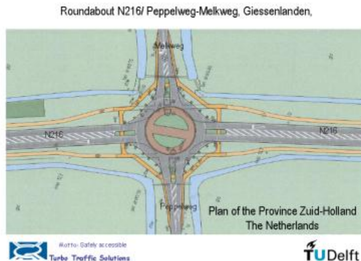
FIGURE 5.25 Roundabout Showing Offset Road through a Roundabout in the Netherlands
