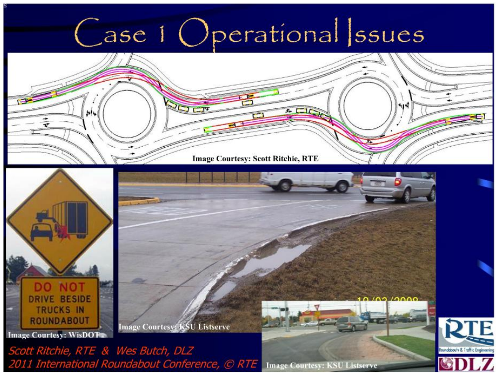
FIGURE 5.20 Operational Issues of Some Roundabouts and Turning Movements
