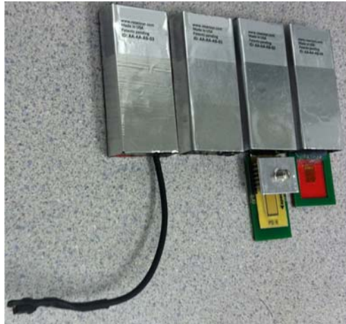
Figure 2: Left to right: SenSpots for humidity, tilt, crack, and strain monitoring.
