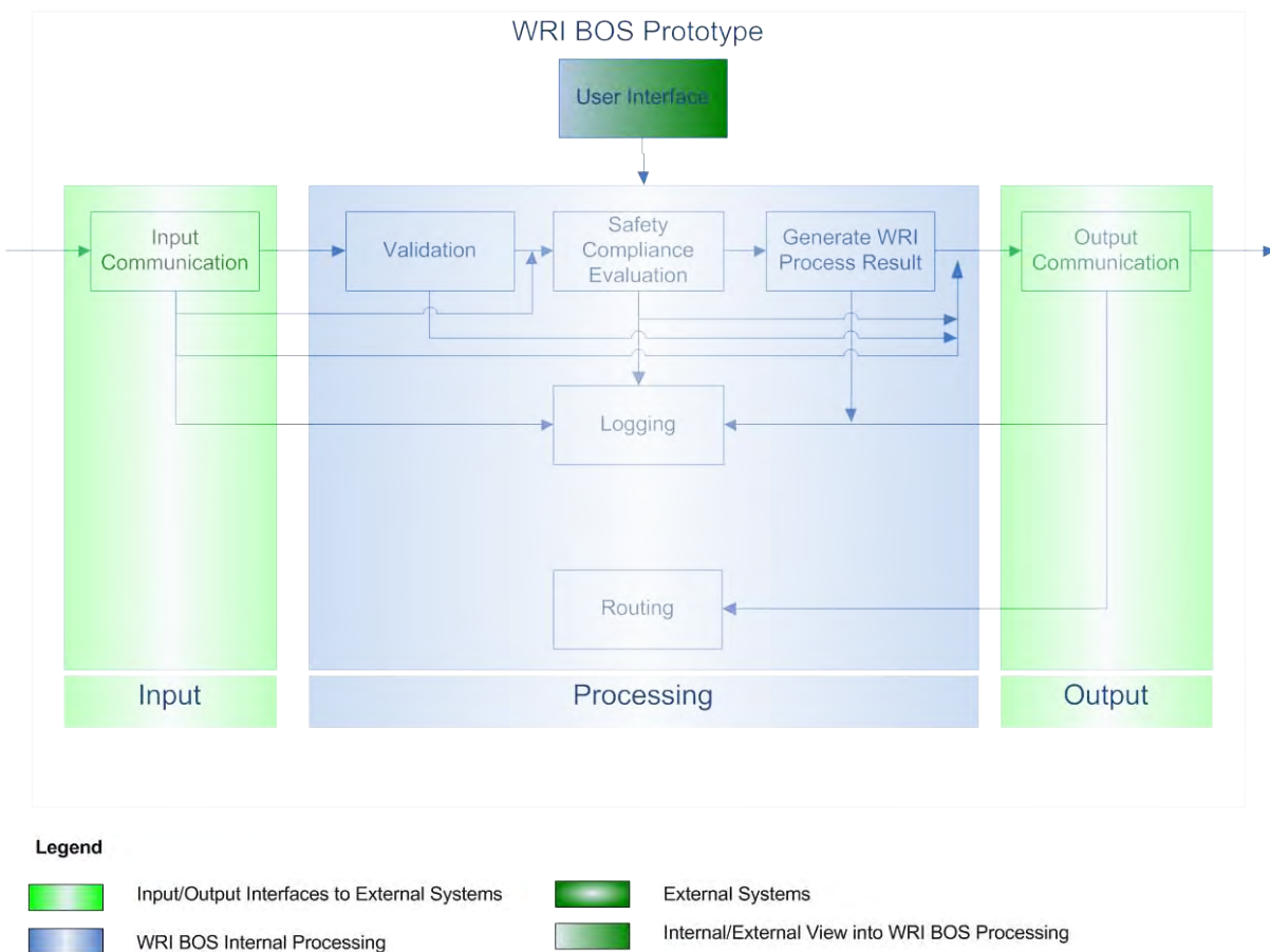
Figure 23. Diagram. GBOS communication and data processing flowchart.
