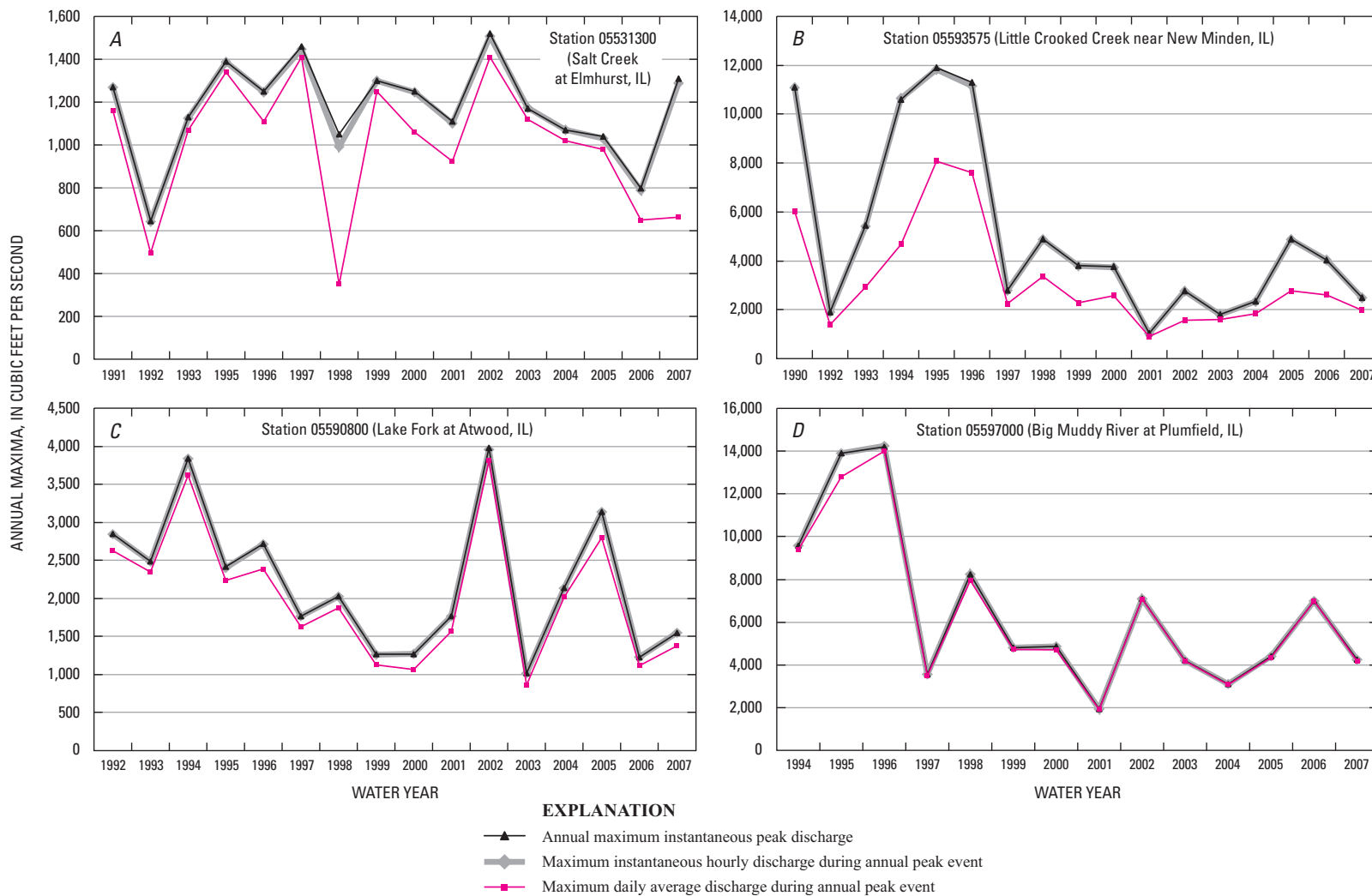
Figure 2.1. Comparisons among annual maximum instantaneous peak discharges and maximum instantaneous hourly and average daily discharges during annual peak event: (a) station 05531300 (Salt Creek at Elmhurst, Illinois), near scour investigation site 1-7; (b) station 05593575 (Little Crooked Creek near New Minden, Illinois), at scour investigation site 8-50; (c) station 05590800 (Lake Fork at Atwood, Illinois), at scour investigation site 5-20; and (d) station 05597000 (Big Muddy River at Plumfield, Illinois), at scour investigation site 9-1. Water years with missing hourly data during the annual peak event are not shown.
