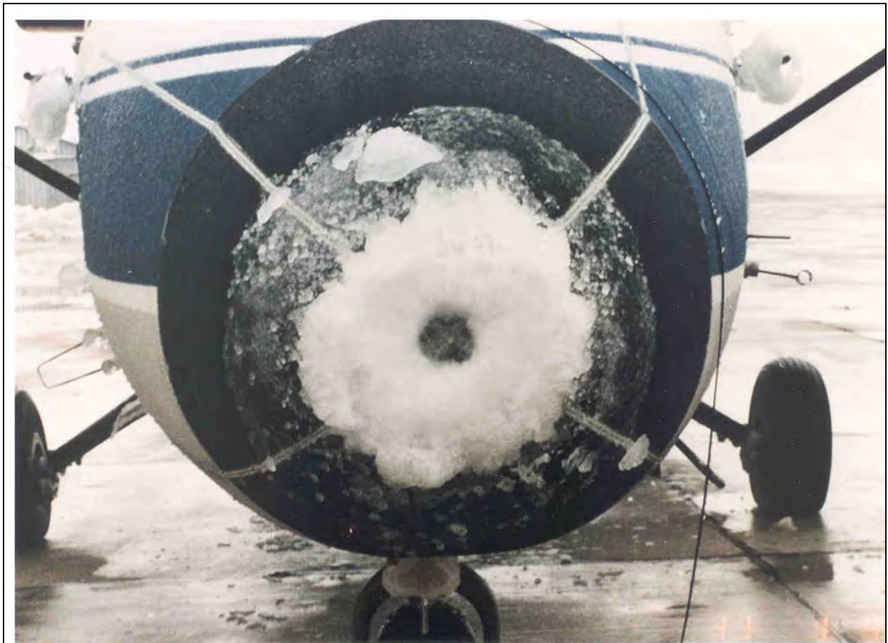
Figure 4. Freezing Rain on a DH-6 Twin Otter (photo courtesy of Porter Perkins, 1992)
