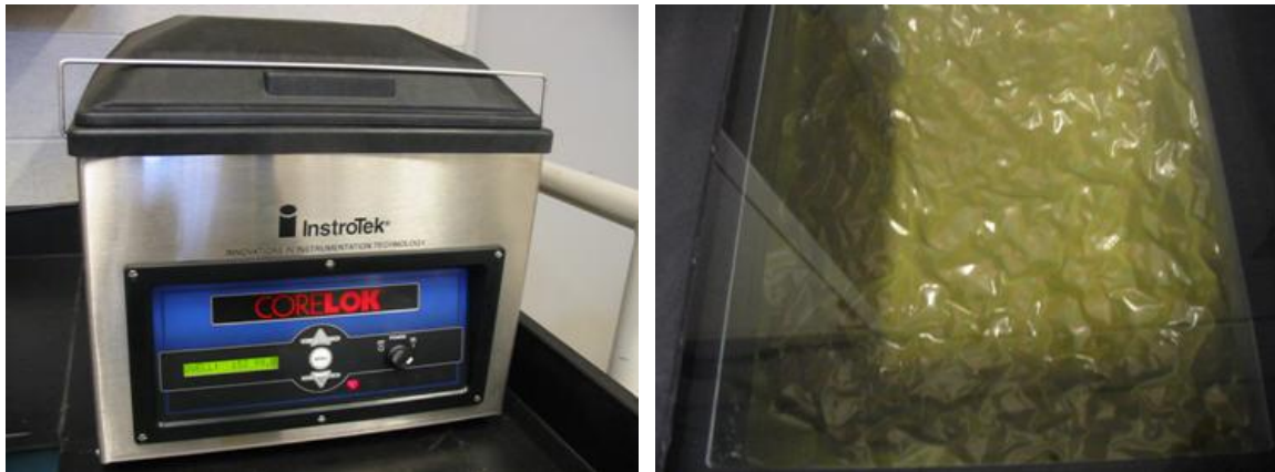
Fig. 5-3 CoreLok Device to Measure Theoretical Maximum Specific Gravity
