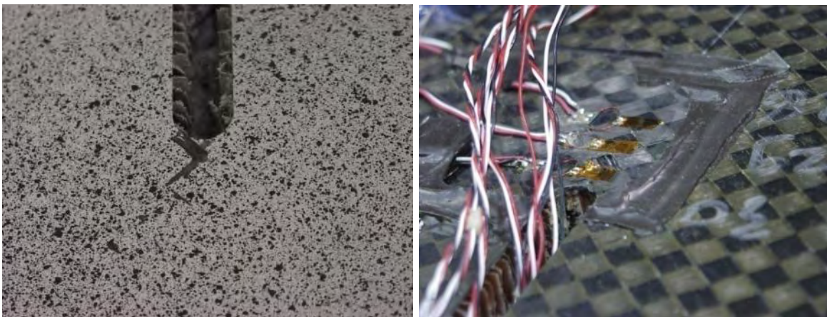
Figure 26. Panel CP4 Extent of Posttest Convex Facesheet Damage
