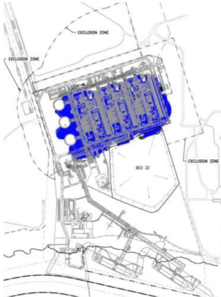
Figure 4.12-3 Vapor Cloud Explosion Overpressure Contours
