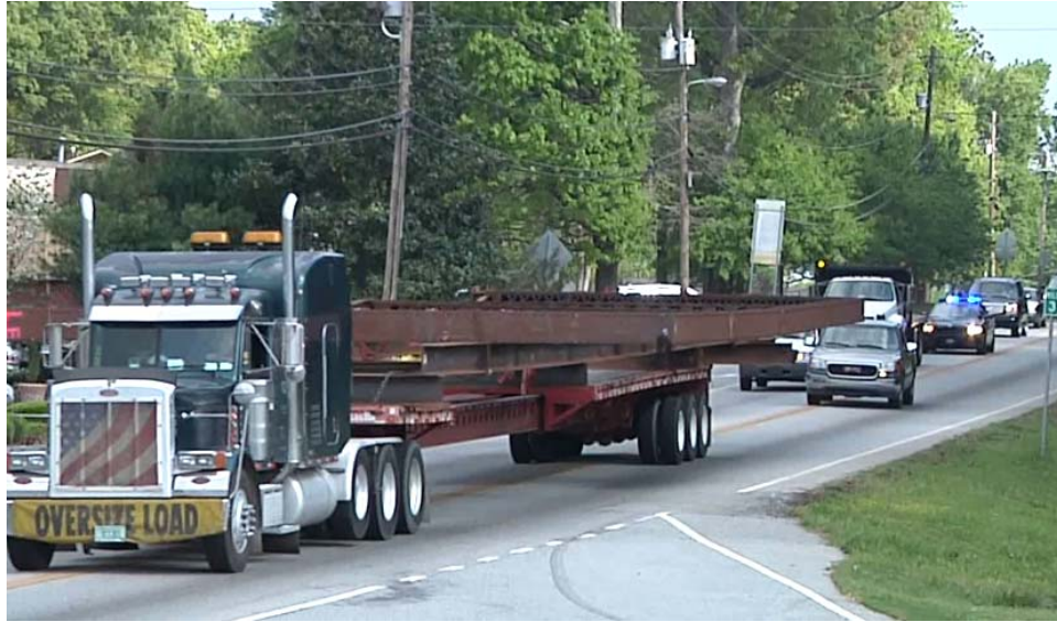
Figure 53. Transportation of one of the planar trusses on S. Hill Street, Griffin, GA, in route to the storage site at the Griffin airport (Courtesy of Sharman Southall, GDOT).
