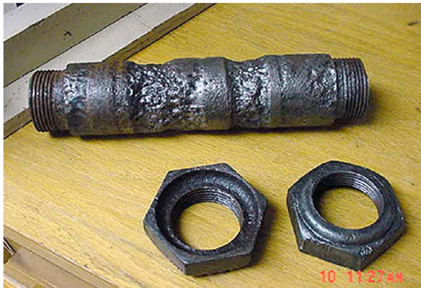
Figure 14. Example of a heavily corroded pin (VDOT 2006).
